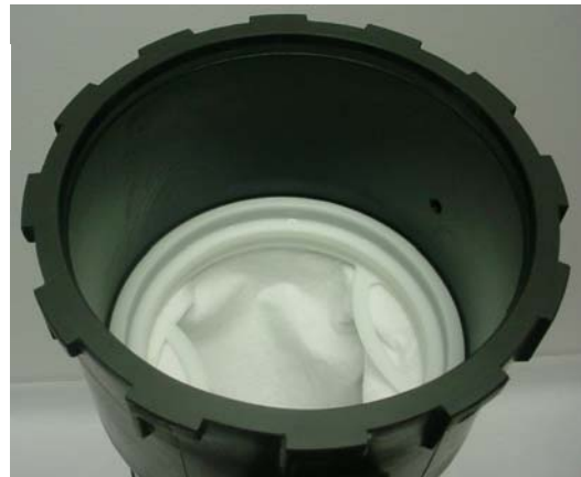
Figure 25 Bag Inserted Into Vessel
